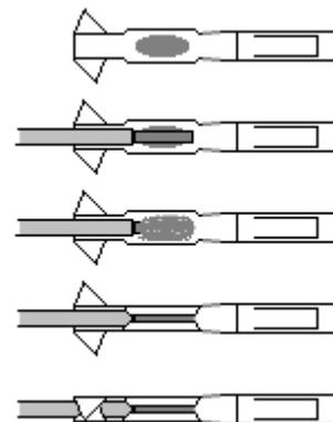
Bend the borders of the channels round with flat pliers. Then bend the plates around the insulation and finally put the sockets in the connector so that the locks would lock on. If there is resistance, gently try to lift the lock on the connector with a tip. Not too much, otherwise it will stay open forever. Lean the tip at the edge of the socket and gently move it forward. You probably used too much tin or bent the borders too little.
