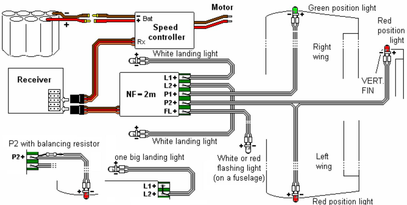
The P2 circuit (red) is calculated to supply series connection of two red diodes, as shown on image. You can connect only one diode, but then it is advisable on the place of the second red diode in the circuit attached ballancing resistance 390Ohmů to provide comparable luminous intensity with the green LED on the circuit P1.
