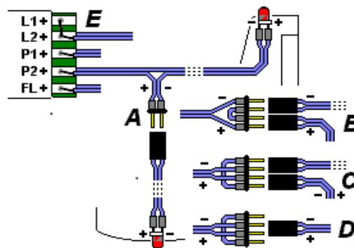
Examples A, B and C in the figure show a possible realization of removable strips. Variant C compared to variants A and B have the advantage that the splitter can involve only a single connector, see Fig. option D (NOTE the polarity, the connector must then be rotated). If you install only one landing reflector, you can increase its shine bridging L1 and L2, as indicated by Figure E. This must be done on the other side of the unit as well.
