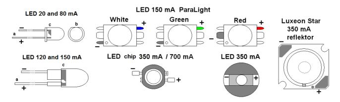
For 20 and 80 mA diodes the positive pole has a longer outlet (a) and the negative pole has a trimmed edge (b) and usually extends inside the body (c) to hold the chip.
