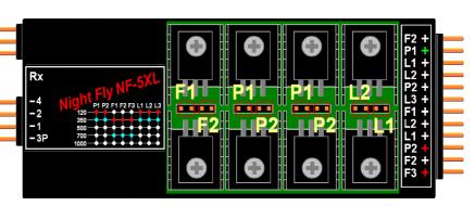
the following picture the positional and landing lights without jumpers have current 120mA with jumper 350. Flash lights without jumpers 350, 700mA with jumper.
