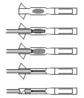
wire and the socket would be in line. If your hand slips, you can heat the wire again and when it gets released, fix it. Keep eye on the solder temperature, you might lose the insulation. Keep the same polarity with all the cables, it is aesthetical. If you e.g. solder the diodes' positive pole on the farther socket, the locks of all connectors will be oriented upwards.
