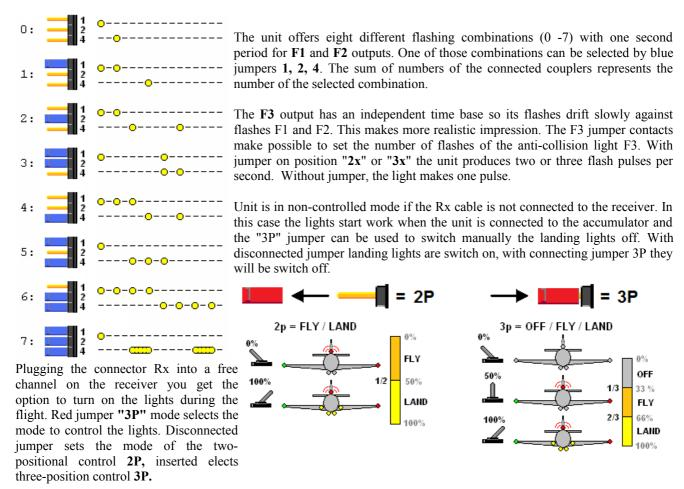
In 2P mode position and anti-collision lights are on continuously and landing lights are controlled from the transmitter. The 3P mode is the standard range of servo divided into thirds. In the first lights are switched off, in the second position lights and anti-collision lights are switched on, in the third all the lights are switched on.
