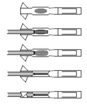
Drop a little tin in the middle part of the socket, not too much. The thin tube tin is easier to dose. Put the wire in the farther socket and heat it so that the tin connects. Then repeat it with the closer socket. See to it that the wire and the socket would be in line. If your hand slips, you can heat the wire again and when it gets released, fix it. Keep eye on the solder temperature, you might lose the insulation. Keep the same polarity with all the cables, it is aesthetical.
