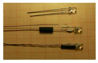
the wire beforehand as far as possible from the intended soldered connection - if you don't do so, they might shrink in a wrong place. After soldering in both stems and cooling pull the insulation on the connection and heat it gently from all sides with the solder so that it would shrink (you need to try it). It is recommended to heat at a place behind the tip where the solder is clean. Thus the insulation will not be littered with tin and resin.
