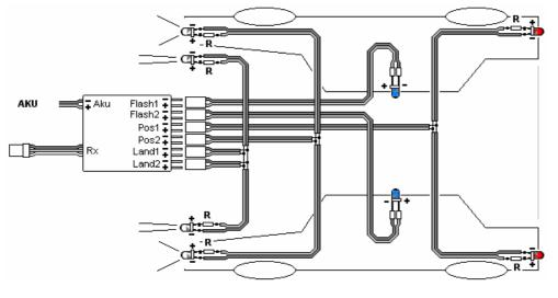
To divide the current in the diodes equally, both diodes in the current have to be the same type and colour, otherwise the diode with a smaller voltage will be alight only.
