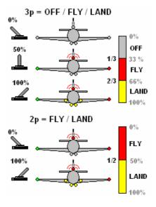
Controlled with a remote controller, anti-collision and landing lights automatically begin to flash when the plane is unable to receive a signal from the remote controller.
