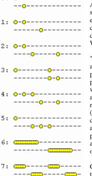
Anti-collision light outputs flash with one second period. Three jumper contacts (1, 2, 4) enable to choose one of 8 flashing combinations. Combination sequence number is determined by the total of connected jumpers. When open, all jumpers make 0.
