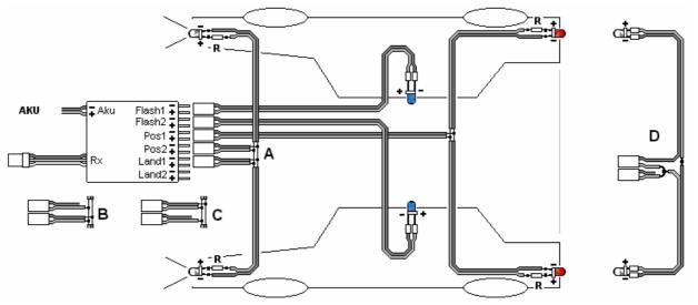
**Note:** In the last scheme shown, lights and headlamps are parallel-connected. However, even in case of a serial light connection a parallel circuit connection is possible; this is shown in the picture D and could be used in case of the first scheme i.e. the car model. Aeromodellers may use it for parallel-connected circuits Land1 and Land2 to reach an effect of gradual turning-on of landing lights.
