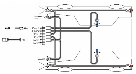
connected to the circuit Land1, representing full beam. This purpose should be taken into consideration while choosing the illumination angle of the diodes. The flash circuits can be set up to a slow flashing or a fast flashing 1:1, using them as strobe lights.
