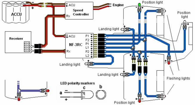
In case there is at least one diode connected to the circuit, the transistor is relieved. The maximum operational voltage of 14V stated in the parameters is in accordance with that (12V transistor + approx. 2V diode). By a bigger amount of diodes in all circuits the circuit can theoretically operate up to the voltage of 17V (twelve-cell). However, the warranty does not apply by such an operation.
