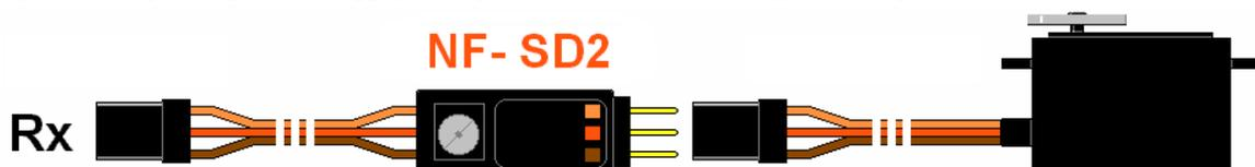
The module is connected to receiver with a Graupner, Hitech type connector. The servo or regulator cable is connected to the output connector on the other side. **ATTENTION**, the output connector is not secured against change of polarity. The order of colors must be kept the same as on the cable to receiver, as is indicated on the first picture. **The same colors must be towards each other, not the other way!**
